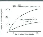
It exhibits protective effect preventing chlorinated ion as well as water absorption on concrete surface.
